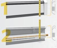
Measure from floor to the top of the existing back plate.
